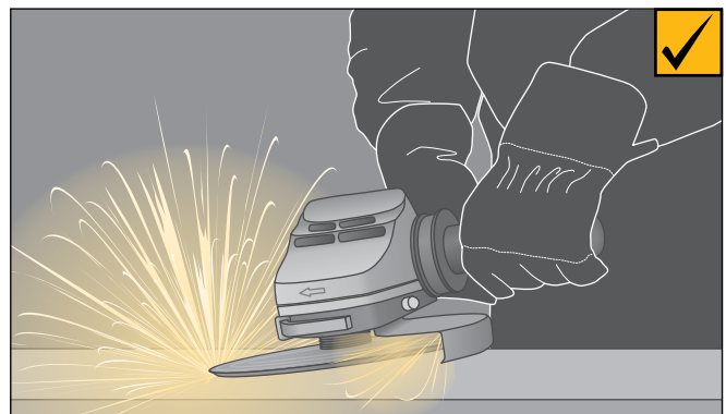
Only use angle grinders for the specific material and purpose for which they are designed.
